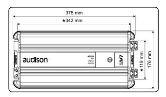
\* Drilling dimensions for fixing
