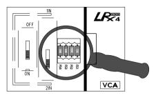
Replace FS1, FS2, FS3, FS4 resistors according to the values in the setting panel table.
