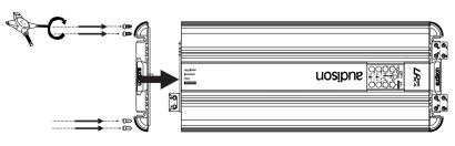
**5** - Mount the plate back by fixing it through the screws; then, re-assemble the transparent cover which protects controls.
