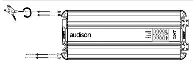
1 - Remove the transparent cover which protects controls and then the 4 screws which block the metal plate by using multispanner.
